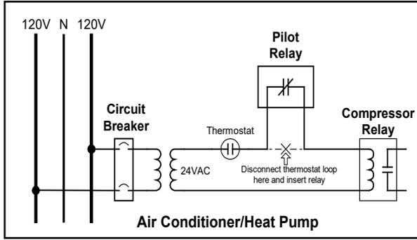
**10.2.2 Controlling the Entire Unit using Low Voltage control:**
